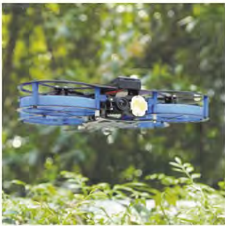
TIM: TREE INSPECTION MICRODRONE DESIGNER Singapore University of Technology & Design / National Parks Board of Singapore (Foong Shaohui, Soh Gim Song, Jake Goh Tze Huan, Ang Wei Jun, Lee Jiong Le, Tan Chee How & Ervine Lin Shengwei)
