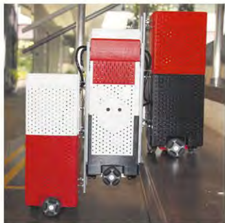
STETRO: A MODULAR RECONFIGURABLE STAIRCASE CLEANING ROBOT DESIGNER SUTD-MIT International Design Centre (IDC) (Manojkumar Devarassu, Mohan Rajesh Elara, Manivannan Kalimuthu, Shi Yuyao, Karthikeyan Elangovan, Veera Jagadheeshwar, Thein Than Tun, Ayyalusami Vengadesh, Pratap Kandasamy) CLIENT National Robotics R&D Programme Office
